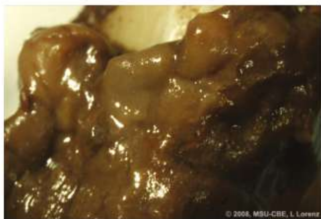
Figure 8. Stereoscope image of inner dispensing tube of a plastic counter-mounted dispenser coated with unknown brown substance. 7.5X.
