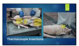
The yellow boxes indicate thermocouple locations: right and left hams, the stuffing, right and left shoulders, and between the shoulder blades.
